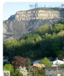
(c) With mountaintop removal, everything lying above an ore deposit is just removed. This controversial mining technique is common in coal mining regions, such as Kentucky above.
