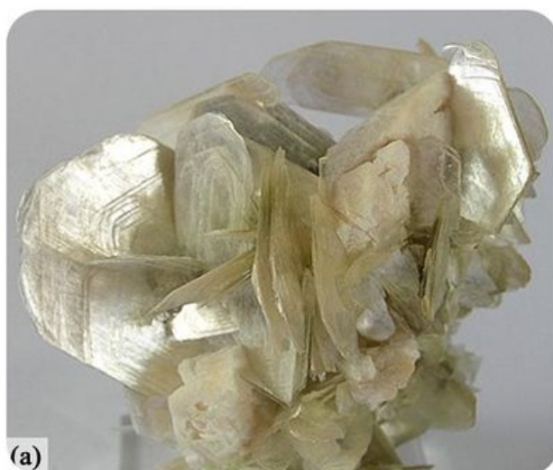
(a) Muscovite has platy cleavage due to the sheet-like structure of the silica tetrahedra.
