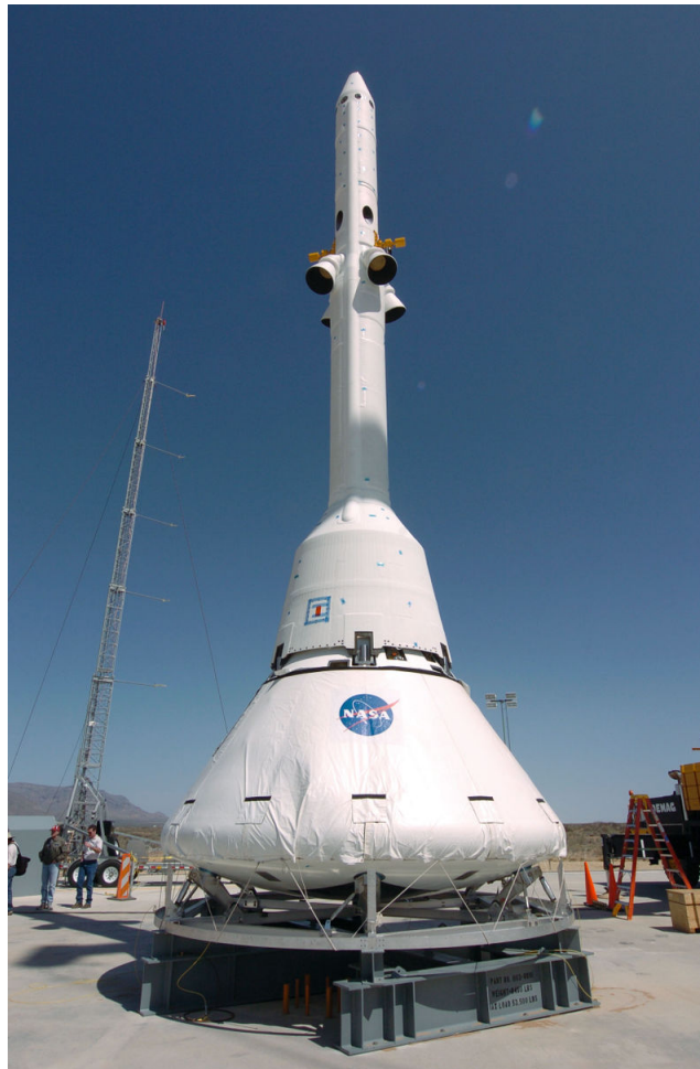
Figure 1: The launch abort system for the Pad Abort-1 (PA-1) flight test is positioned on the launch pad in preparation for the test at the U.S. Army's White Sands Missile Range in New Mexico. The uncrewed, integrated flight test will evaluate the ability of a launch abort system to pull an astronaut crew to safety in the event of an emergency on a launch pad. (Attribution: NASA)
