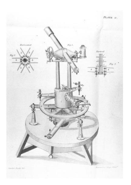
FIGURE 12.3 An old surveyors telescope *theodolite*.
